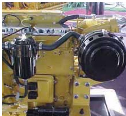
Pictures below: (bottom right) Cummins QSM11 marine engine with CCV cutaway. (below) Caterpillar 3196 marine engine with Racor CCV/AF System.
